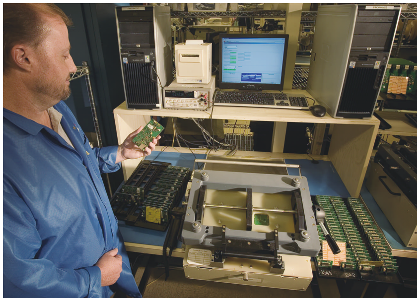
Engineer Chuck Polley examines a test fixture for which he developed the Pogo-pin interface.
