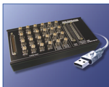
DT9834 Series High-performance, up to 32 channels @ 500kHz
