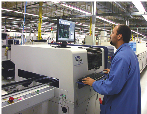
An AOI system performs pre-reflow inspection on an SMT assembly line. Courtesy of MC Assembly.
