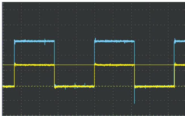
FIGURE 1. Shown here is the waveform of a driver programmed to drive 1.5 V under both no-load (blue) and load conditions (yellow). With a 6- \Omega load condition, the voltage at the device under test reaches only 710 mV.
